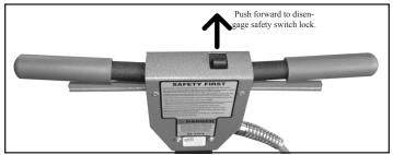
To stop the machine, simply release the triggers. The safety switch lock will automatically return to the engaged position.
